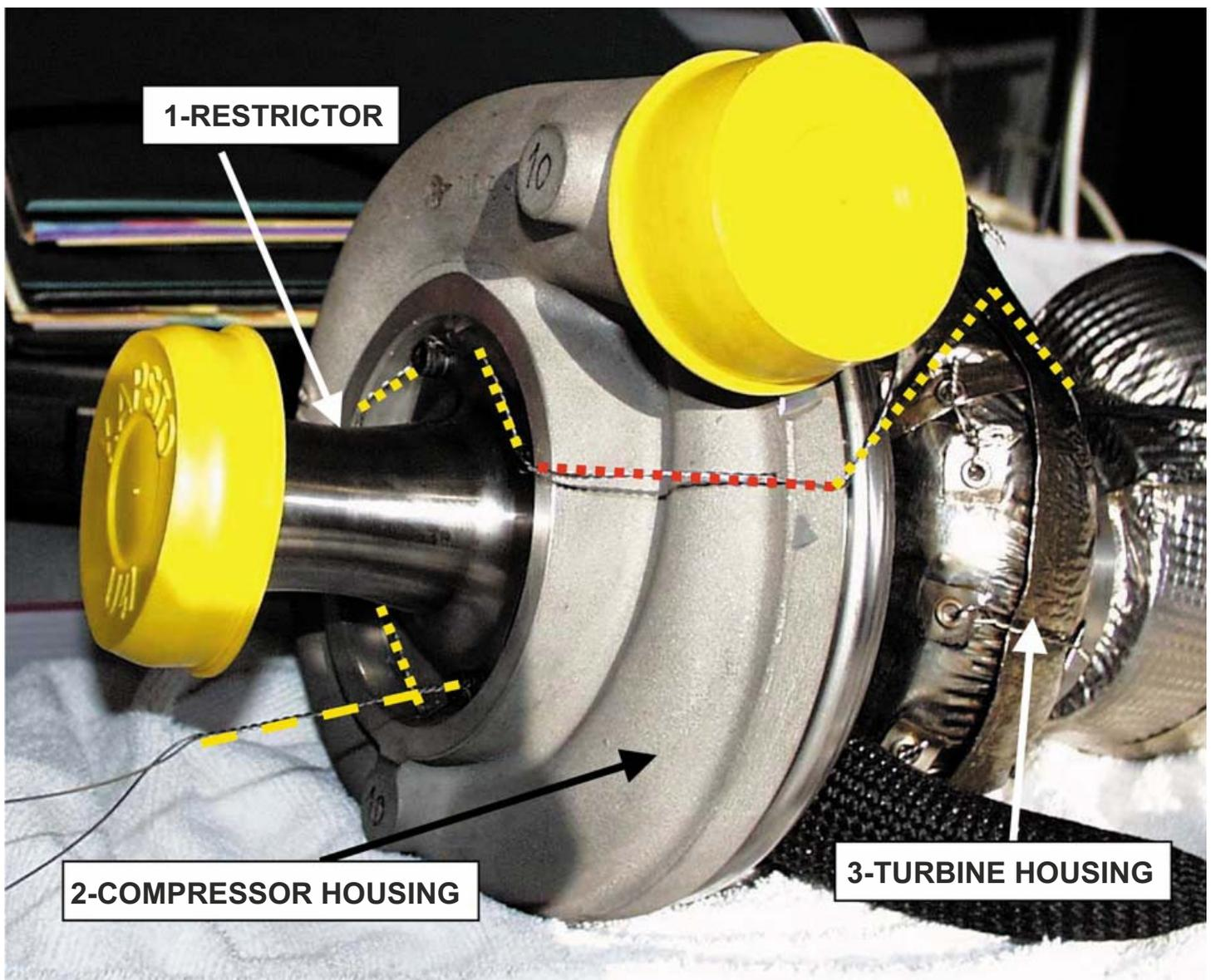
The articles 254-6.1 (Group N) and 255-5.1.8.3 (Group A) from Appendix J state: The restrictor must be made from a single material and may be pierced solely for the purpose of mounting and sealing, which must be carried out between the mounting screws, between the restrictor (or the restrictor/compressor housing attachment), the compressor housing (or the housing/flange attachment) and the turbine housing (or the housing/flange attachment) (see drawing 254-4).
